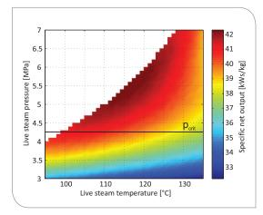
Depending on the external boundary conditions, calculations for local or integral cycle data can be determined. This makes it easy to analyze the sensitivity of influencing variables and cost-effectiveness.
